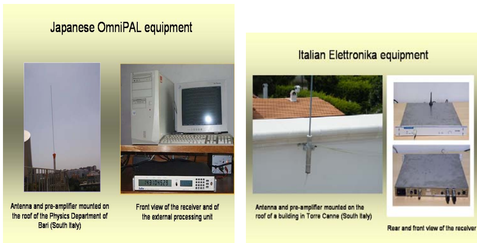
Figure 2: The Japanese OmniPAL receiver and the Italian Elettronika receiver
